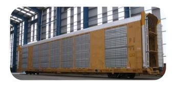
Automax II<sub>®</sub> is a fully integrated, two-unit railcar design with unmatched security. The MultiMax™ rack features adjustable decks for both BI and TRI level service without adding or removing decks.
