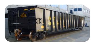
**Gondola Cars** used in for aggregate service. Also used for scrap, debris, raw steel, and various structural items
