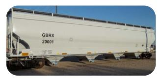
Large Covered Hoppers for plastic pellets, petrochemical products, distiller dried grains or other light-density products.
