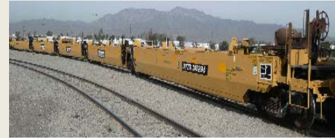
Type: 5-unit 40' well with 125T Intermediate trucks Fleet distribution: 40' DTTX
