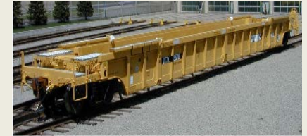
Type: Single-unit 53' well with 70T trucks Fleet distribution: 53' DTTX
