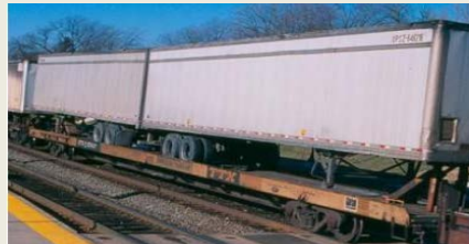
Type: Single-unit 89' All- purpose (RTTX) Fleet distribution: CONV
