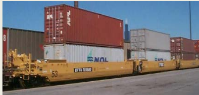
Type: 3-unit 53' articulated well with 125T Intermediate trucks Fleet distribution: 53' DTTX
