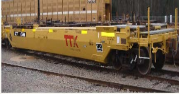
Type: Single-unit 40' well with 70T trucks Fleet distribution: 40' DTTX
